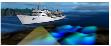
Figure 1: Graphic of a NOAA vessel conducting a hydrographic survey utilizing a multibeam echo sounder. For more information on surveying techniques visit
