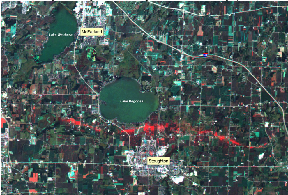
“After” image Satellite map of tornado path from the Stoughton, WI Tornado of August 18, 2005 composed of satellite imagery from Landsat TM and Terra ASTER showing damage path in red.
