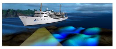
Figure 1: Graphic of a NOAA vessel conducting a hydrographic survey utilizing a multibeam echo sounder. For more information on surveying techniques visit
