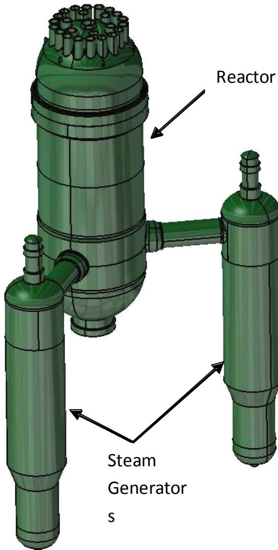
The nuclear supply system module is based on a 625 MW thermal (MWt) annular reactor core in a large steel reactor vessel. It is a two-loop system with the reactor connected to two parallel steam generators and helium circulators.
