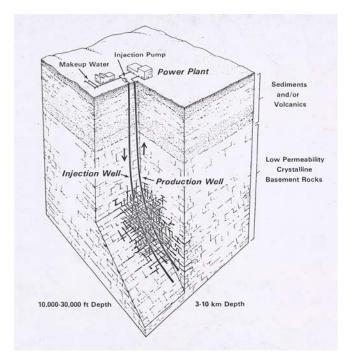
Figure 3. Schematic of a conceptual two-well enhanced geothermal system (EGS) in hot rock, in a low-permeability crystalline basement formation. Connectivity has been established by hydraulically stimulating the rock contained between the injection and production wells.
