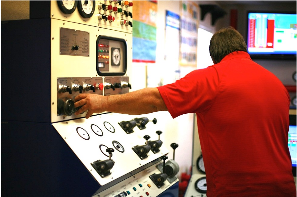
Figure 3. Well control simulator at UBATC in Vernal, Utah.
