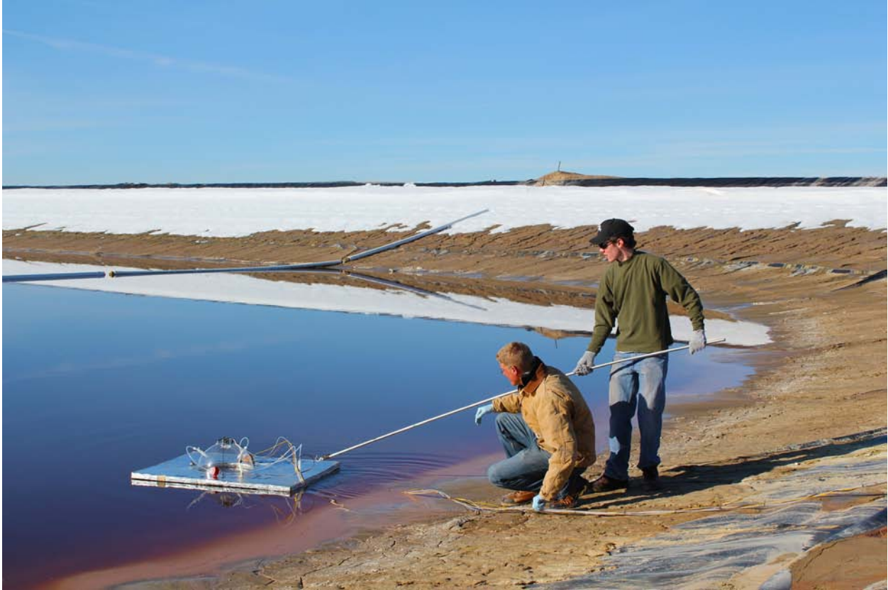
Figure 4. USU students deploy an emissions measurement chamber on a produced water pond in the Uintah Basin.
