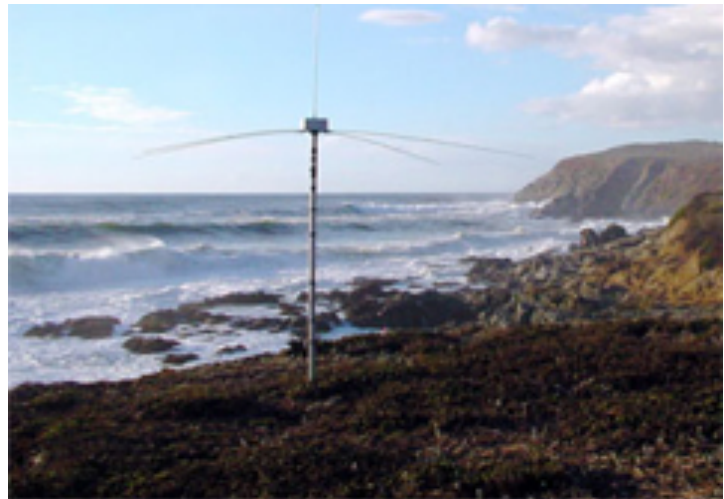
Figure 3. High frequency radar receiving antenna, used for measuring speed and direction of ocean surface currents in near real time. http://www.ioos.noaa.gov/hfradar/
